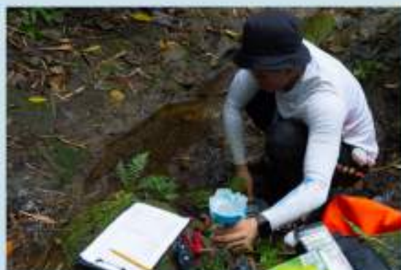
Figure 7. Measuring of water quality using a water quality multiparameter in Arillo estate.
