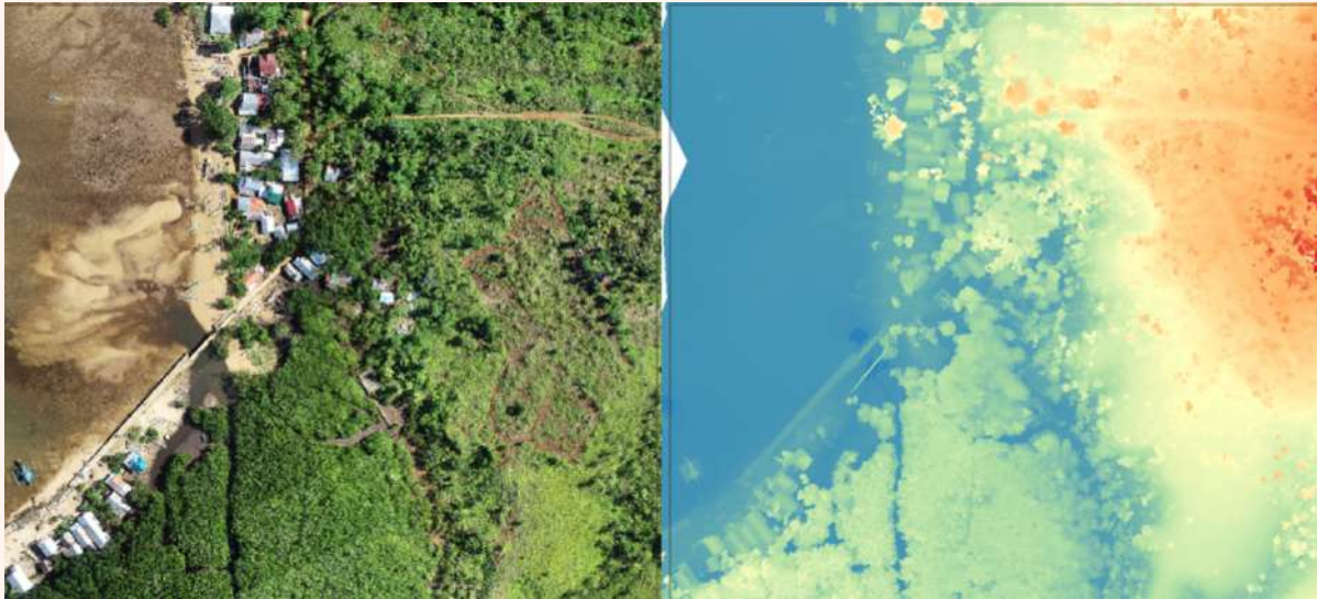
Figure 8. Sample orthophoto mosaic image (left) and Digital Surface Model (right) processed using DJI Terra software. This flight data acquisition is located at barangay Pamosaingan in the Municipality of Socorro.
